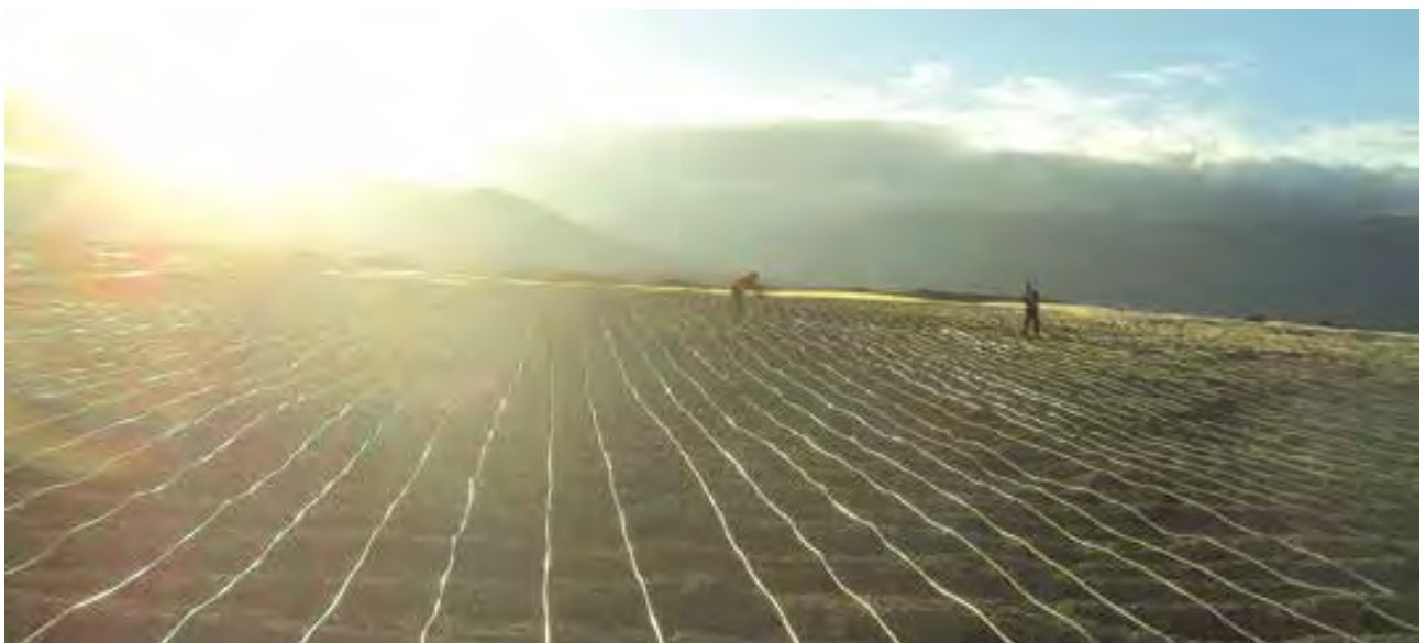
Above: Leach Pad irrigation system (© Xstrata Copper)
